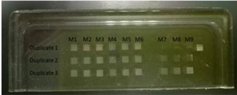
Patterned moulds on 2mm x 2mm area
