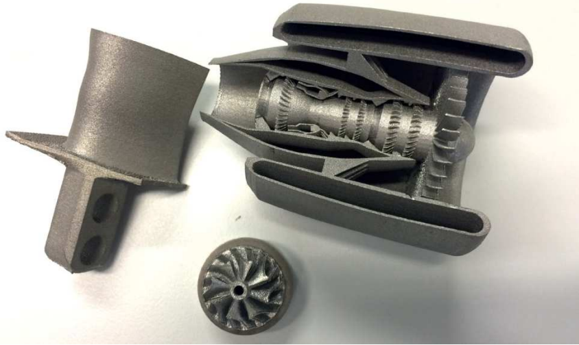
Aerospace components manufactured with selective laser melting
