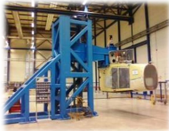
TIGER HELICOPTER ASSEMBLY LINE MATING JIG
