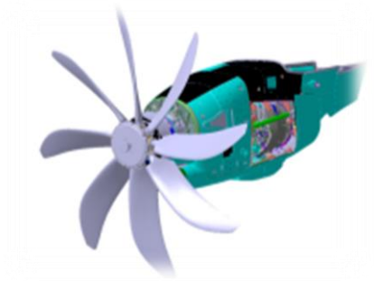
AIR INLET DUCT (ATF) FOR TP400-D6 DEVELOPMENT ENGINE
