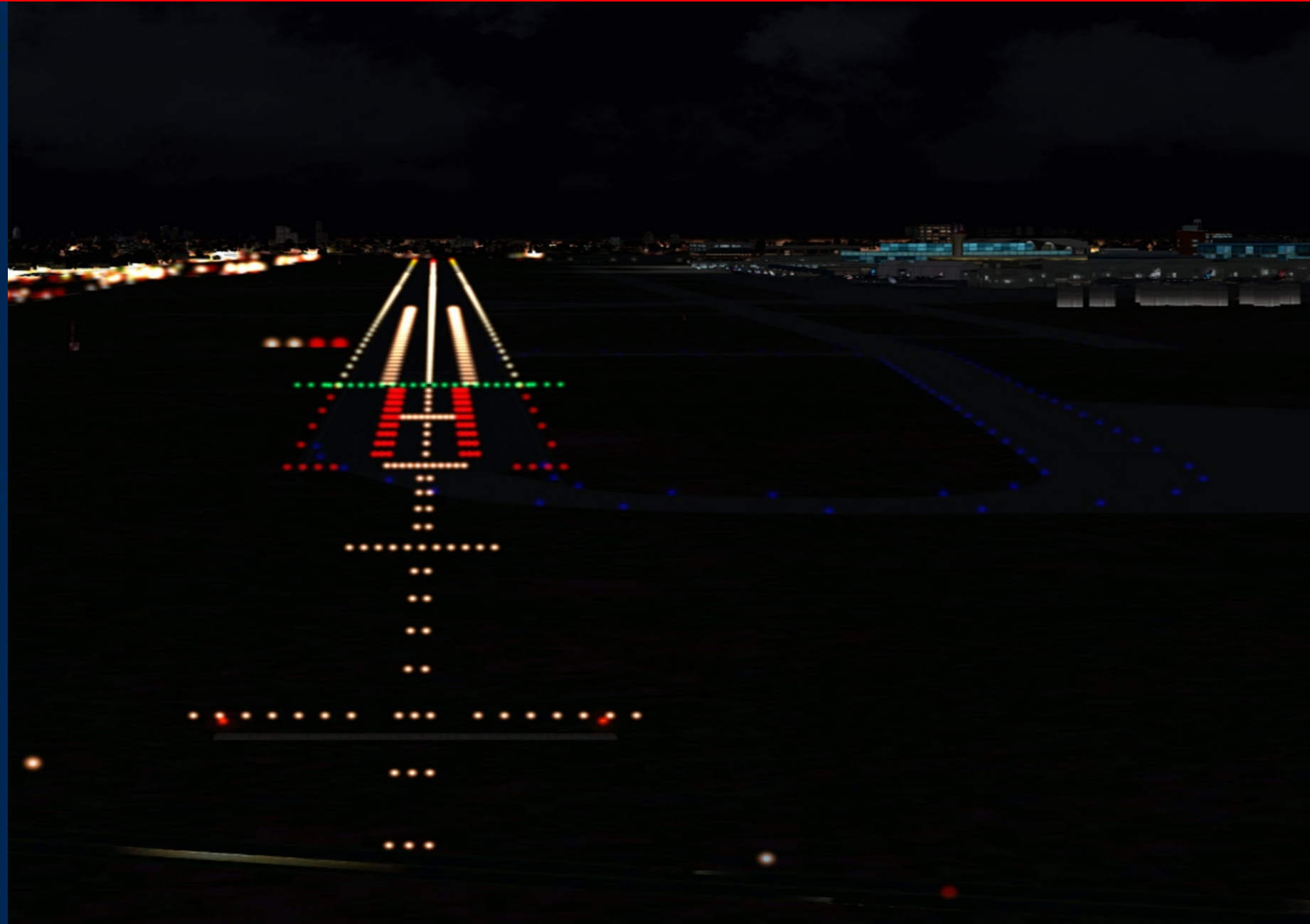
APPROACH AND RUNWAY LIGHTING TYPICAL CAT II OR CAT III SYSTEM
