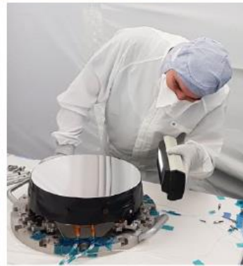
EQM IRS M1 M4 Set up for Vibration Test Campaign
